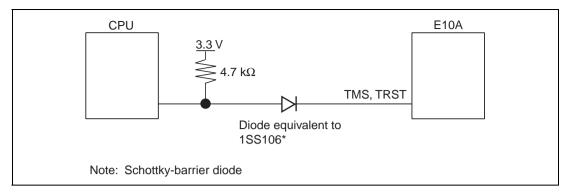
Figure 1.4 Countermeasure against the Leakage Current in the Emulator
